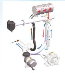
The QAL 182 WS utilises direct extractive heated sampling which can be configured to either extract an isokinetic sample or extract a sample based on a pre-set user-defined velocity. The extracted sample passes directly into a heated vaporising chamber. The sample is superheated and exits into a controlled sample chamber. The *ProScatter*® sensor provides a high accuracy, high resolution measurement meeting ELV's of 15mg/m<sup>3</sup> or less.
